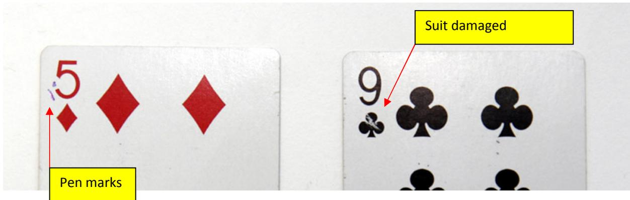
Such damages can make card recognition impossible – this problem can be solved by rotating the card in the Feeder by 180deg so the machine will try to read symbols on the opposite corner (hopefully without damage) and continue dealing or discard such damaged deck.
