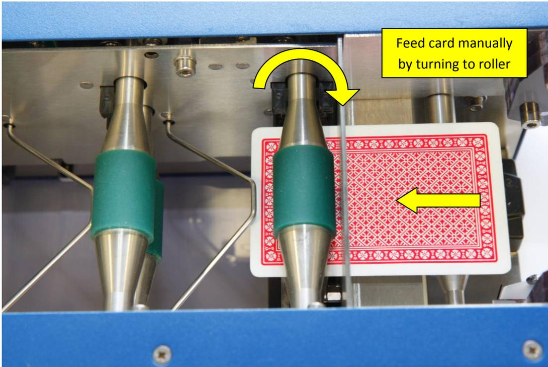
Insert card manually, and check the clearance between the gate and the card. In the lower position the gate should be around 1mm below the card. In the raised position the gate should be around 2mm above the card.
