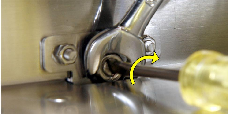
5. Using the 8mm spanner to lock the locking nut:
