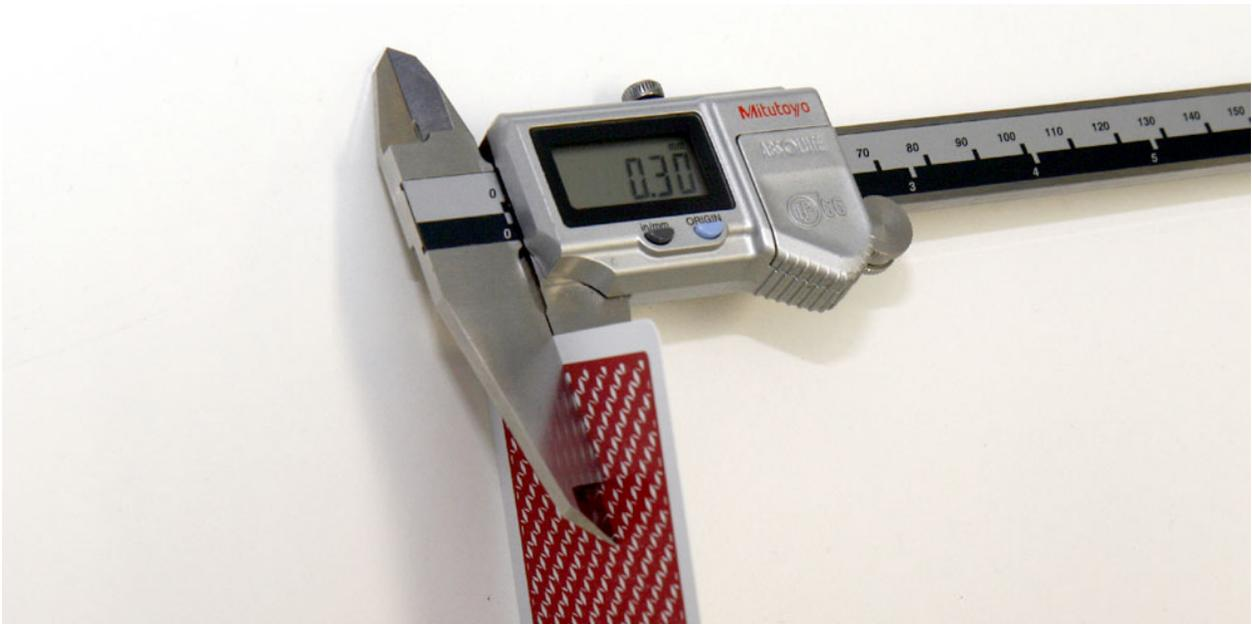
If a vernier caliper is not available it is possible to measure card thickness using a standard ruler. Hold a full deck (52 cards) and measure thickness as shown below. Then divide the result by 52. This gives the thickness of a single card.
