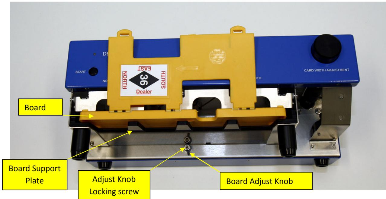
To adjust the Board Pocket, a 3.0mm Alan key is required. The Board Pocket adjustment is performed by rotating the Board Adjust Knob located under the Board Support Plate:
