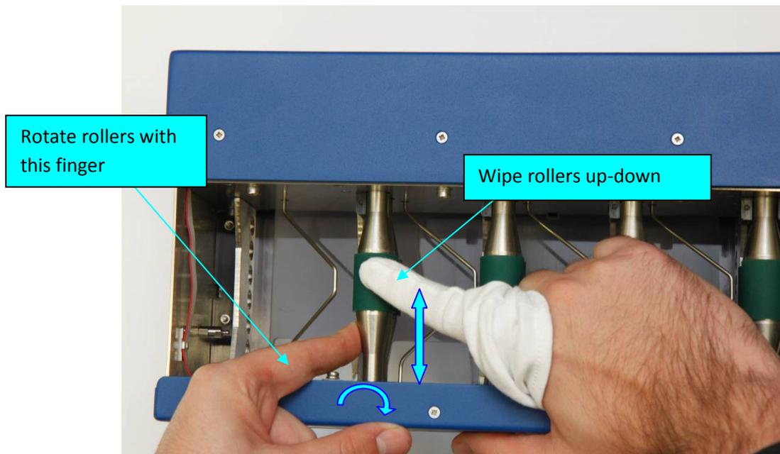
4. Similarly clean the bottom roller. When the top roller is rotated the bottom will rotate also, thus during cleaning it is easier to rotate the bottom roller by rotating the top one.
