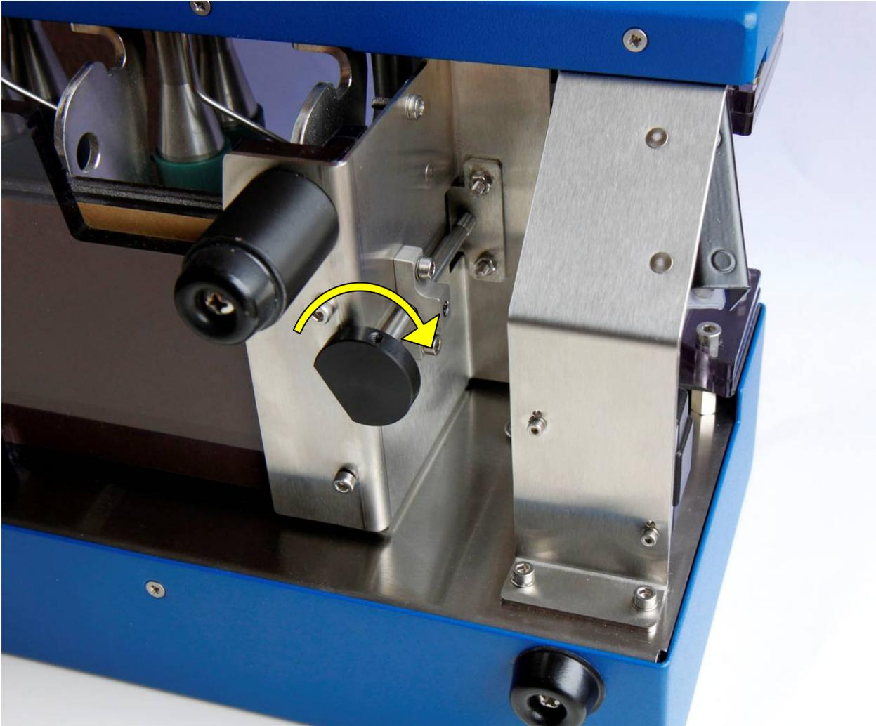
4. Tighten the locking grub screw to lock the mushroom in position.
