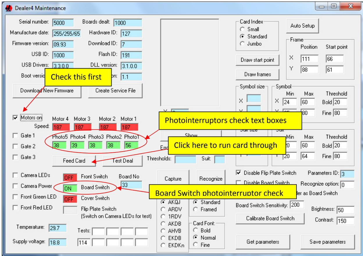
Not every dirty photointerruptor problem can be observed on the “Maintenance” screen. The photointerruptors should be cleaned if frequent Gate Errors (Error number: 1 to 8 or 17 to 24) or Card Jam Errors (Error number: 9 to 16) occur despite the “Maintenance” screen not showing any problems.
