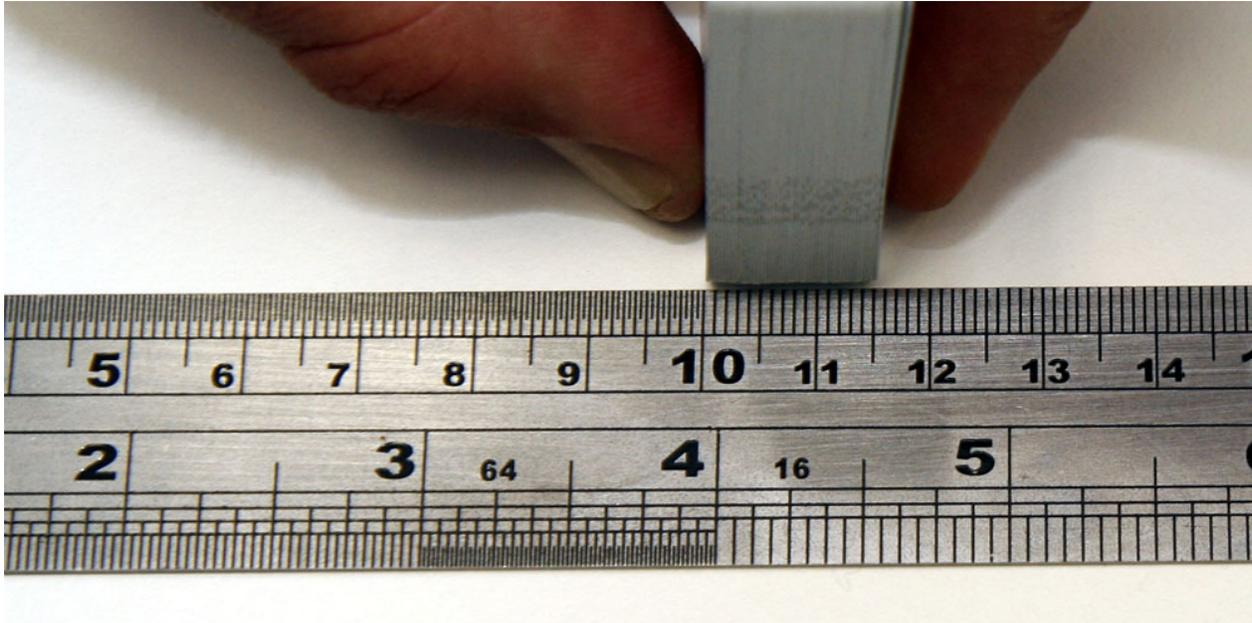
If card thickness is known the correct gap size can be calculated by multiply card thickness by 1.2 to 1.4.
