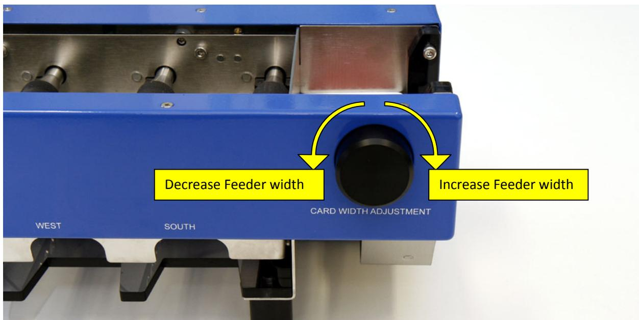
To adjust the card width, put one card into the Feeder and by turning adjustment knob set the adjust plate to touch the card on side:
