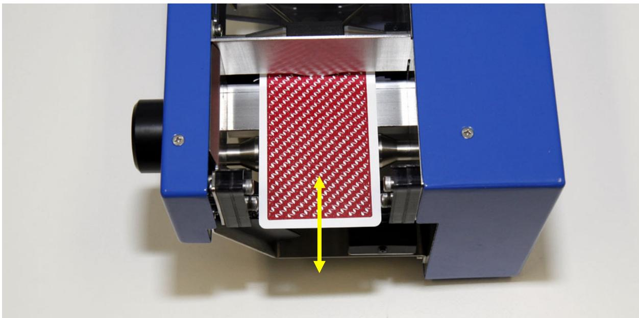
2. While the first card is still in the Feeder Gap try to fit a second one into the gap. This should be not possible. If the second card can fit into the gap even only slightly it means that gap is too large.
