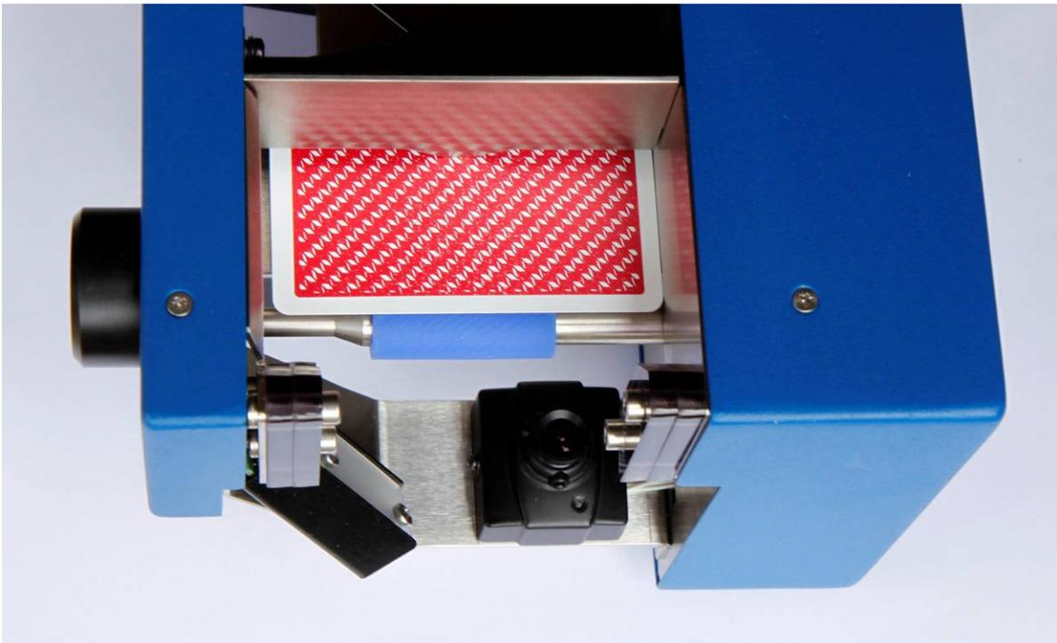
3. Rotate the Bottom Mushroom Knob clockwise until the mushroom touches the card in such a way that the card cannot be moved by hand. Do not over tighten. Then rotate the Knob a 1/4 turn counterclockwise. Use flat part of the knob to define a 1/4 turn:
