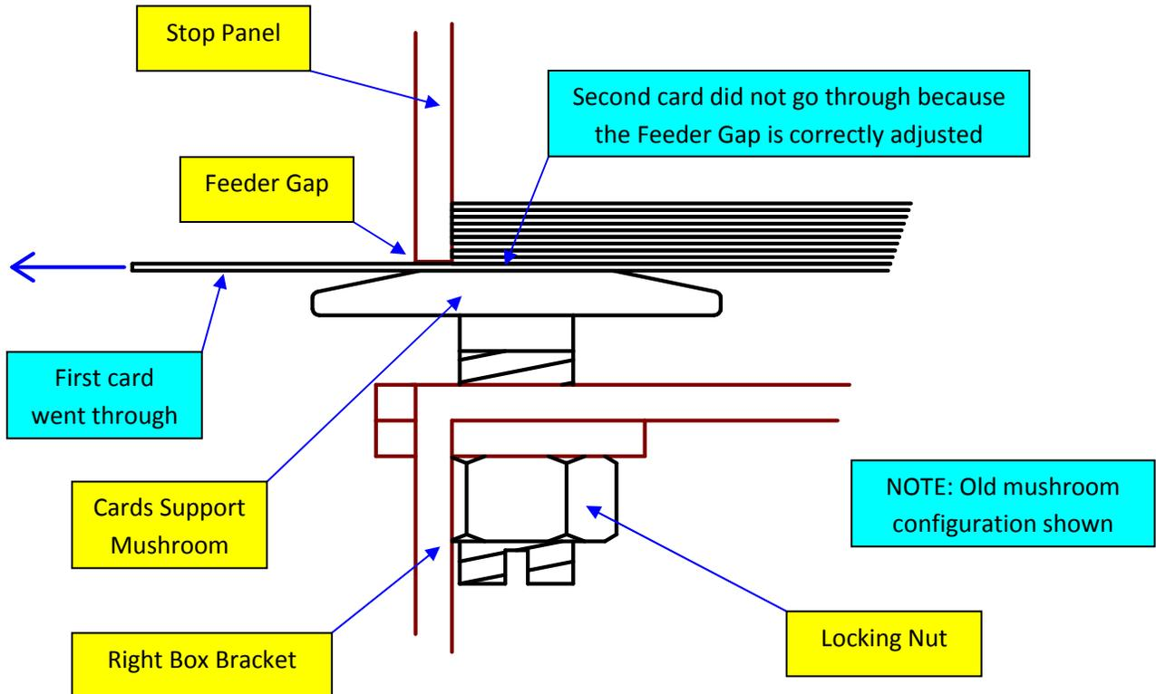
The correct Feeder Gap size is essential for proper Dealer4 operation. If the gap is too small it will be difficult or impossible to fit the cards through the gap. If the gap is too large two cards can through at the same time or the second card can block the first card.
