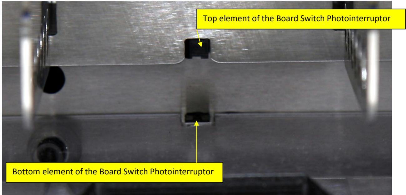
If any of the photointerruptors are too dirty the light beam can be blocked and Dealer4 will not operate correctly.
