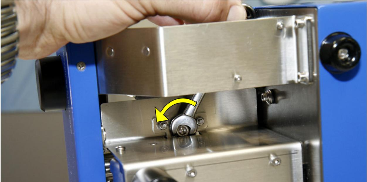
3. Put the Feeler gauge blade with the desired thickness into the Feeder Gap. If the blade does not fit (Feeder Gap is too small) rotate card support mushroom anticlockwise (when looking from the bottom) using a small flat screwdriver. This makes the gap bigger and will allow the Feeler Gauge blade to fit. Some early models (serial numbers from 4001 – 4012) are fitted with a card mushroom without a screwdriver slot. In this case the mushroom has to be rotated by hand.
