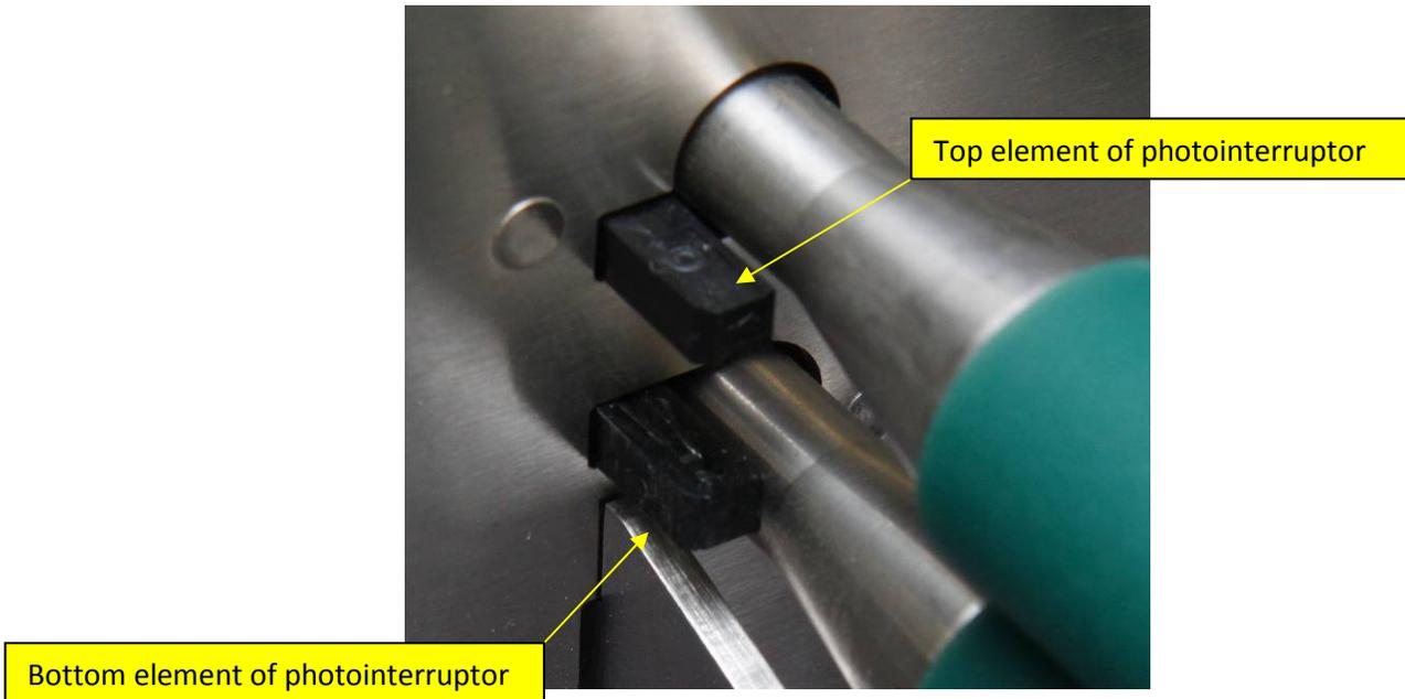
The photointerruptors play an important role in the dealing process. There are five photointerruptors in the machine on the left side of each roller pair and one more on the right side of the first roller.
