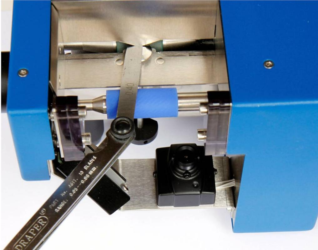
3. With the Feeler Gauge blade in this position rotate bottom mushroom knob clockwise until it touches the blade. Do not use too much force in this step – if the mushroom is rotated too much the Feeler Gauge blade may become difficult to remove. The Feeler Gauge should be tight in the gap but possible to remove without too much force.
