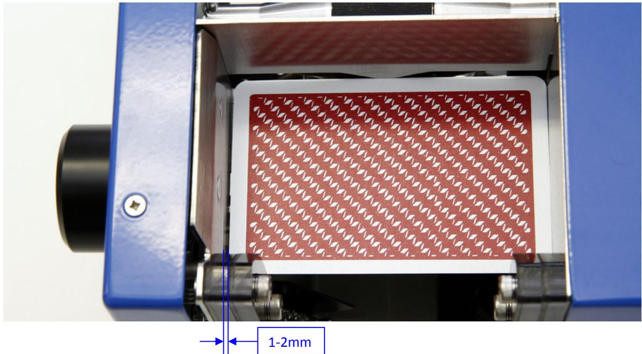
It may be necessary to adjust the Feeder width every time a new type (size) of card is used.
