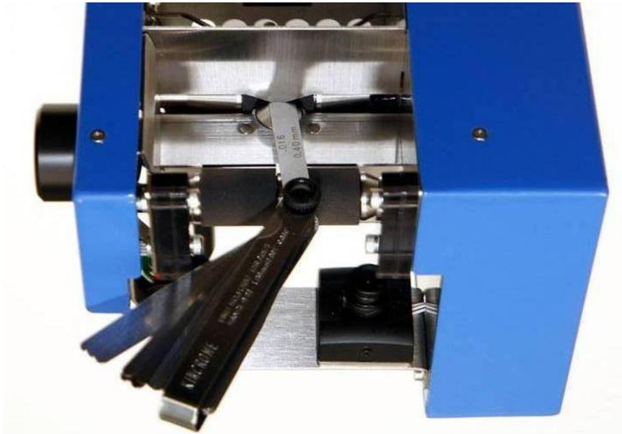
4. With Feeler Gauge blade in the position shown above, rotate the mushroom clockwise until it touches the blade. Do not use too much force in this step – if the mushroom is rotated too much the Feeler Gauge blade may become difficult to remove. The Locking nut should be held by a spanner during this step to not disturb the rotation of the mushroom
