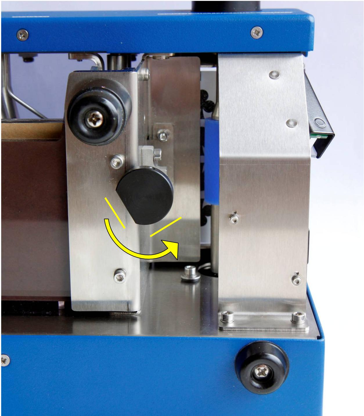
4. Now tighten the locking grub screw to lock the mushroom in position.
