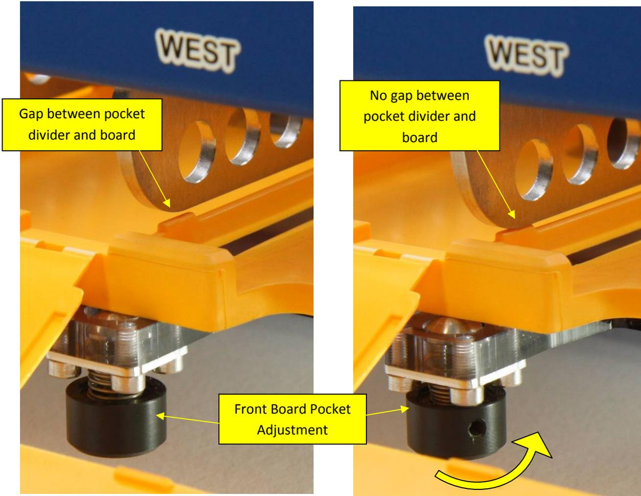
Turn the Adjustment knob until the board touches the pocket dividers. Do not over tighten.
