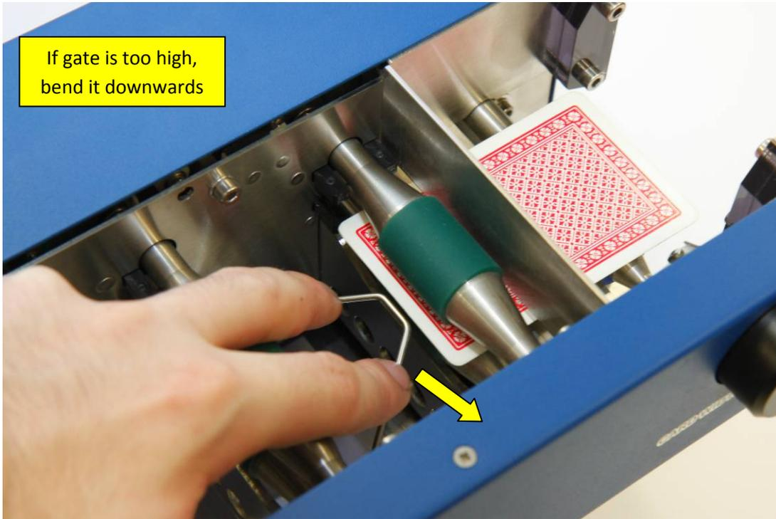
If the gate is too high, bend it downwards. Bending the gate about 10 mm downwards should be enough.
