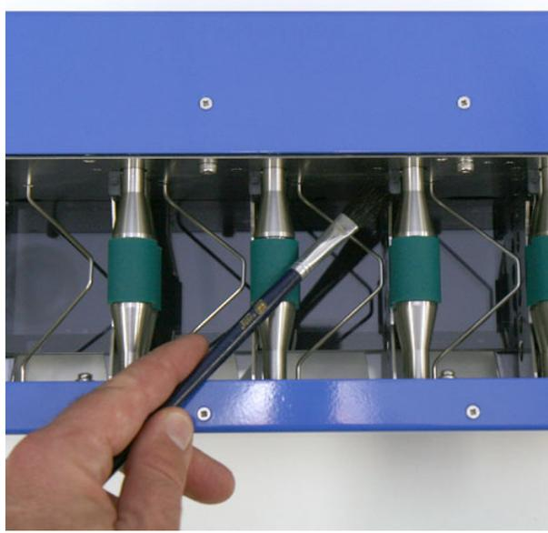
The best access to clean the first photointerruptor is from the Feeder side:
