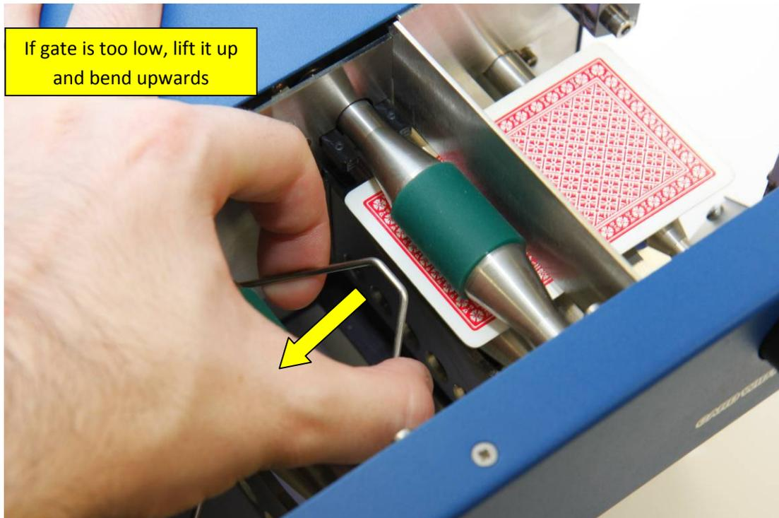
If the gate is too low, lift it up and bend in the upwards direction. The gate will have to be raised about 10mm.
