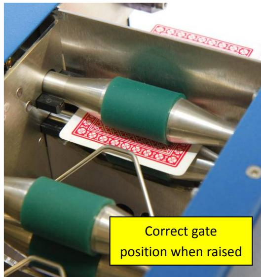
4. Once a problem gate has been identified, disconnect the machine completely and gently bend the gate as required.
