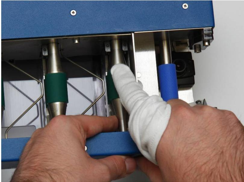
6. Cleaning the first bottom roller is the most difficult part. Rotate the top roller and clean the bottom one from the left side. Be careful not to bend the wire gate which directs cards into the "South" pocket.
