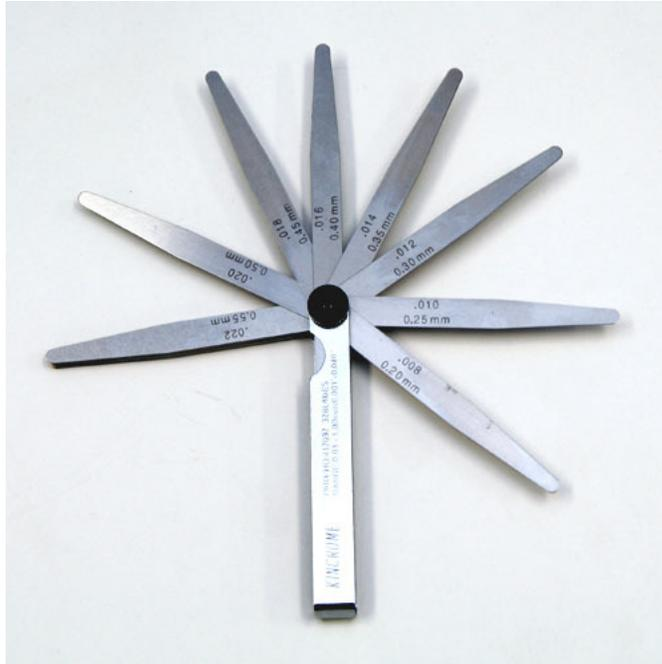
To measure the gap try to fit blades one by one into gap starting from thickest one until it will fit into gap. The thickness of this blade is the size of the gap. Compare this measurement with desired gap size.
