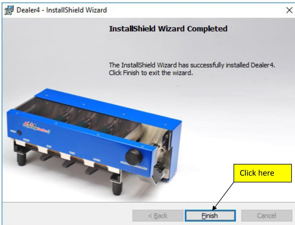
7. Now it is time to connect machine for the first time. Connect the machine using the USB cable provided to any USB port available on the computer. Windows will finish USB drivers installation and Dealer4 is ready to use.
