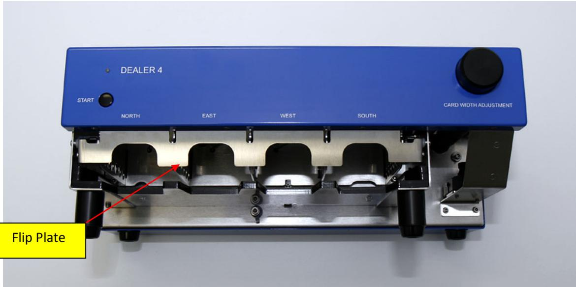
The Flip Plate will not disturb normal card dealing or card box inserting. If access to the cards inside machine is required e.g if card jam occurs, the Flip Plate can be opened (flipped up) as shown on the picture below
