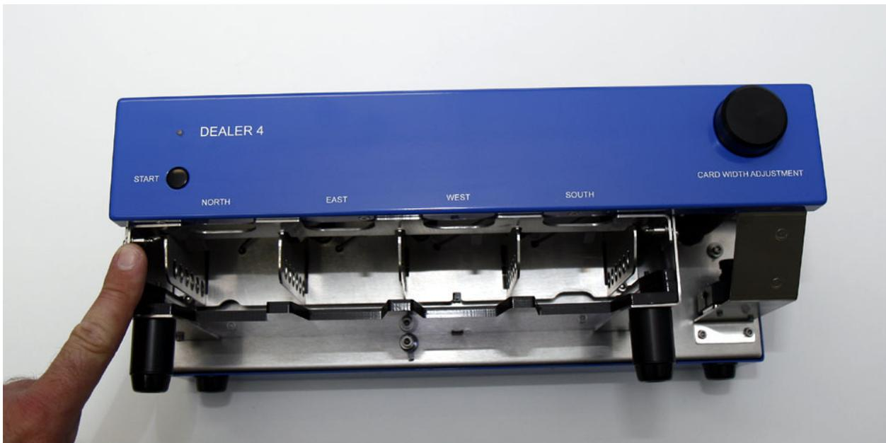
It is not possible to deal with the Flip Plate in the open position. Machine will detect such condition and display an error:
