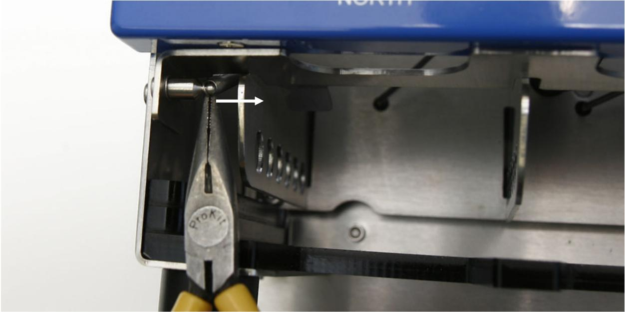
After removing the springs from the top tab remove them from the bottom and take them completely out of the machine.
