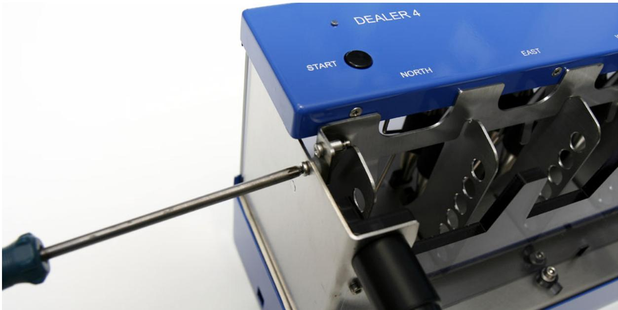
There are two plastic washers on that screw – they can fall down during this operation – it is OK. Find them and put them in a safe place (together with the springs) because they will be needed if the Flip Plate is to be re-attached.
