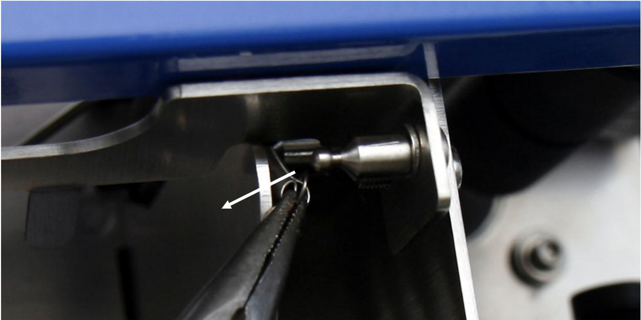
4. Unscrew Flip Plate holding screw from the Left Box Bracket:
