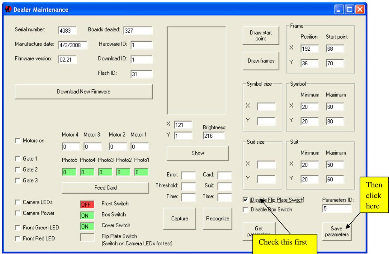
Check “Disable Flip Plate Switch” and then to save this setting into machine click “Save parameters”. If parameters are saved correctly following screen appear:
