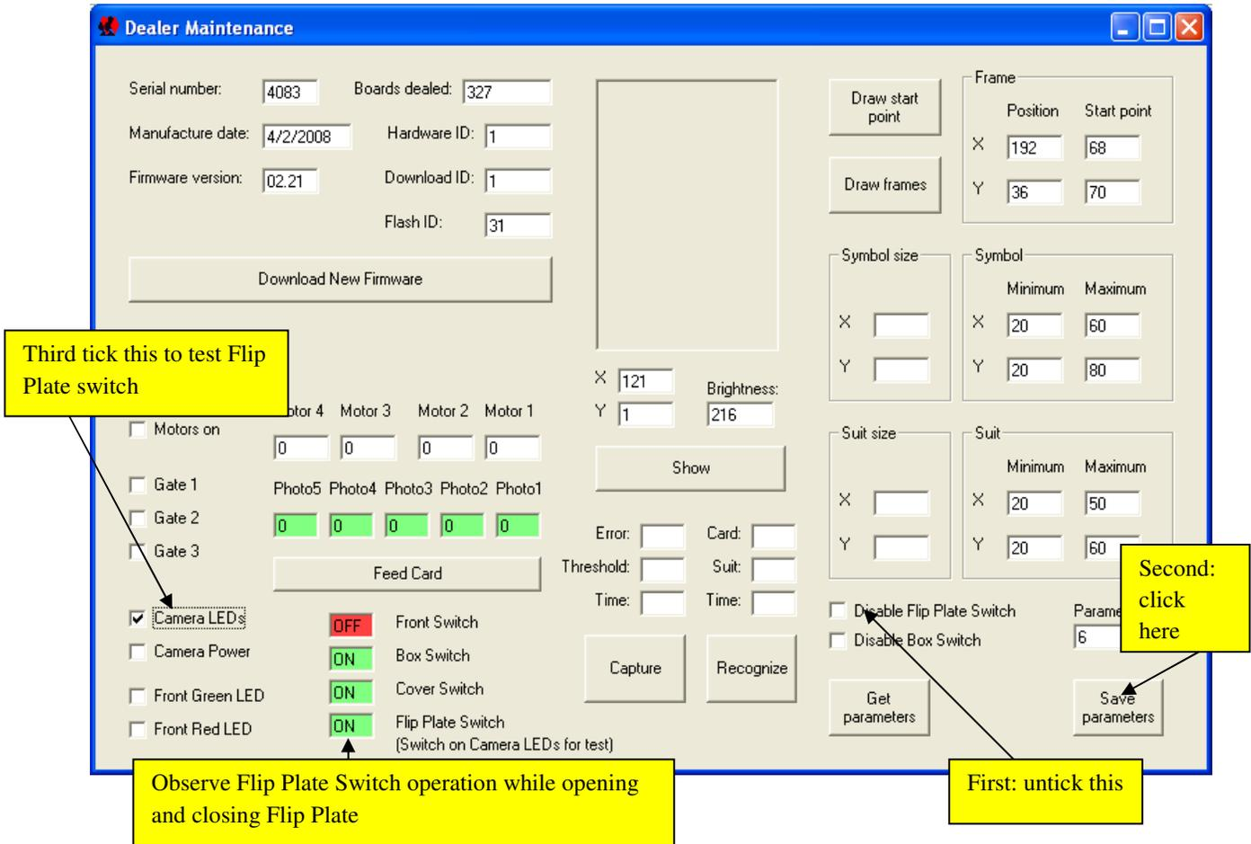
Untick “Disable Flip Plate Switch” and click “Save parameters” to save this change into machine. This step is very important. **Without it, the machine will be allowed to deal with the Flip Plate open which will end up in very nasty card jam.** It is possible to test Flip Plate switch operation by ticking “Camera LEDs” and observe Flip Plate Switch box while opening and closing the Flip Plate.
