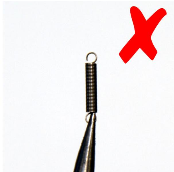
It is important to hold spring on the very end of the pliers tips – otherwise will be impossible to fit end of the spring onto the tab.
