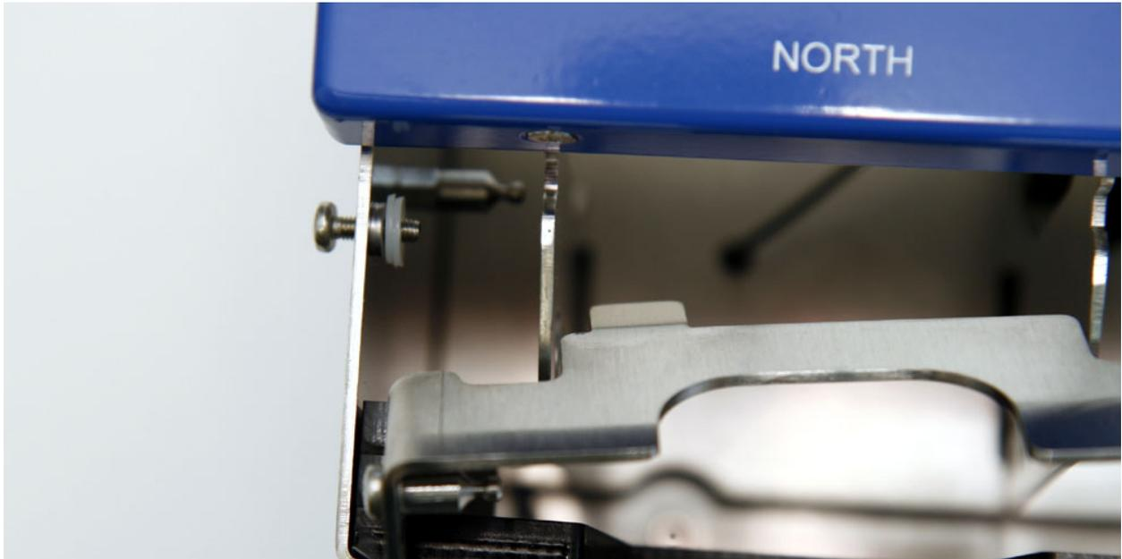
4. The next step is to put Flip Plate into the left screw. This can be little more difficult because of the plastic washer which can fall off during this procedure. If plastic washers are too difficult to attach then the Flip Plate can be fitted without them. Plastic washers provide smoother operation of the Flip Plate but it will still work without them.
